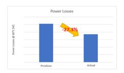
Figure 3: Power loss reduction achievements for the new inverter by DANA TM4 using state of the art Infineon components.
