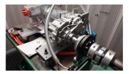
Figure 8: FITGEN Prototype #1 (transmission and motor-inverter group, stand-alone and mounted on the test-bench, courtesy of FITGEN consortium).
