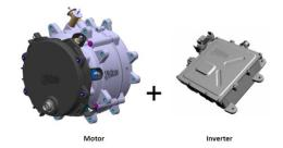
Figure 2: VALEO developed a high power 48V DMG (Direct gear Motor Generator) associated with a power inverter based on MOSfet. A specific power module with GaN transistors in parallel and a dedicated driver have been designed for technology evaluation.
